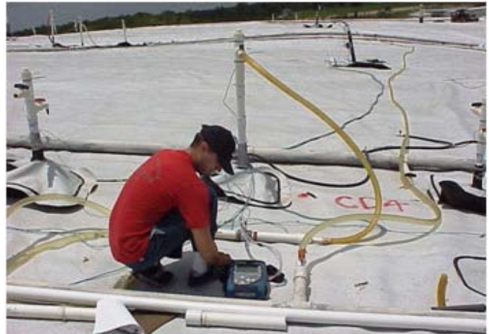
During the air injection experiment, temperature of landfilled waste and air flow rate per well were monitored. If the temperature approached a limit, air flow rate was reduced.
