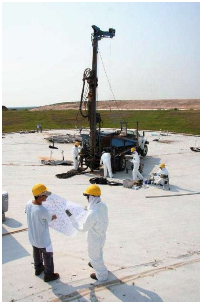
Performance of the bioreactor operation was verified by drilling and sampling landfilled waste. The samples were collected from different areas and depths and were examined for moisture content and degree of biodegradation.
